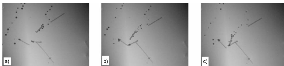
Figure 4. Translational movement of glass fibers 19 at a) 0 s, b) 65 s, c) 145 s (average speed = 1.6 \mu\text{m s}^{-1} ). Dimension of the video frame is 1000 \times 720 \mu\text{m} .
